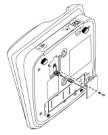
Figure 5 - Mini-SIM Compartment.
